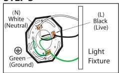
Connect (push) electrical wires from fixture into correct inserts. Black (live), White (neutral), Green (ground)
