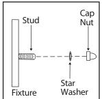
Tuck electrical wires into outlet box and position fixture over studs on mounting bracket assembly. Secure fixture in place with star washers and cap nuts.
