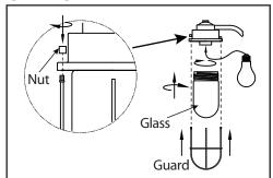
Install the proper bulb type and wattage (not included). Screw glass cylinder on to the fixture. Install the guard with the nuts.
